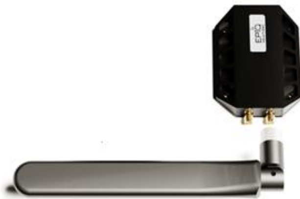
Figure 37. Epiq Solution's Prism scanner and omni-directional antenna (detached).
